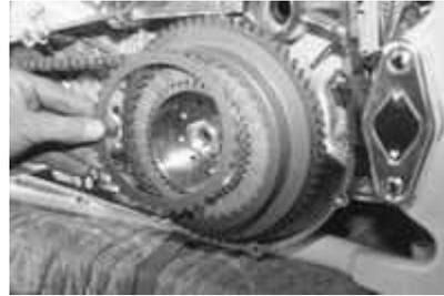
**14.** Install 9 hole pressure plate, use only 6 springs and shoulder bolts. Tighten bolts until they bottom out, this is the correct procedure. The other 3 springs and bolts may or may not be needed depending on how much spring pressure is needed.
