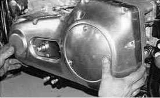
**Fig. 12 Install outer primary cover with gasket**
