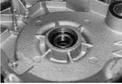
Freeze sealed bearing and re-heat area around bearing housing, the bearing should fall into place without a problem. Replace retaining ring.
