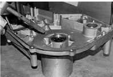
If you are going to remove the stock bearing and use the sealed bearing , then remove primary, remove retaining rings and heat area around bearing for removal.
